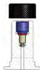
Model of valve stem integrated 5/8" 18 UNF (D)
