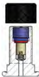
Model of valve stem integrated 7/8" 14 UNF (C)
