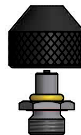
Model of valve stem 7/8" 14 UNF (B)
