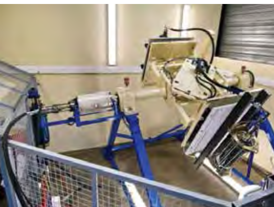
Accumulator test bench for wind turbine application.
